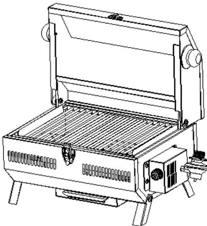
Screw the portable regulator into the side of the control box. Do not over tighten.
