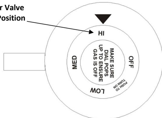
If the burner does not light before 4 seconds of clicking, turn the regulator to the OFF position and wait 5 minutes for the gas to clear before trying again.
